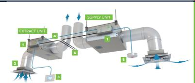
An Ecosmart system combines systems into a simple package, saving space but also time spent installing and commissioning. Alternatively, we offer 'Basic Control' – a simple terminal box for supply and extract fan motor wiring for interfacing to custom-built control panels (by others).
